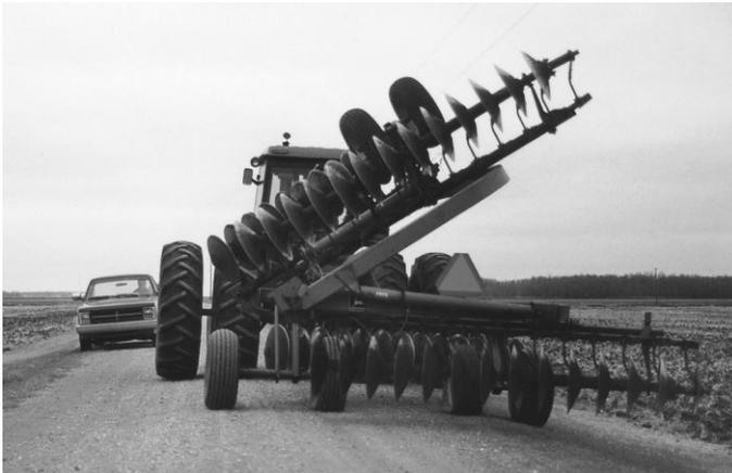
Clearly, farm implements are not designed for travel on public roads. Their size and slow speed make them a hazard, not only for motorists but also for the operator. Compare the dimensions and operating speed of farm equipment and a typical road vehicle, and the problem is evident.
