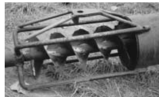
HAZARD: Unguarded grain auger.
