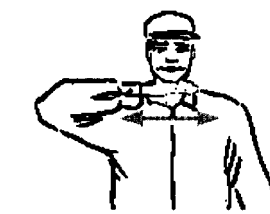
STOP THE ENGINE – Move your right arm across your neck from left to right in a “throat-cutting” motion.
