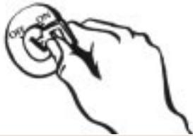
**FACT:** Vibrations from an idling tractor can slip the transmission into gear and cause a run over.
